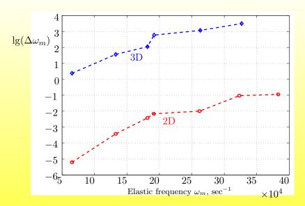
The graph has been calculated for fused silica mirrors with fixed volume
